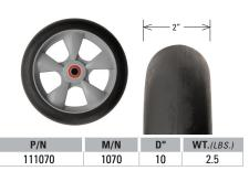
Puncture resistant, non-marking, microcellular tire on one-piece high-density, interlocking polyethylene hub with semi-precision bearings.
