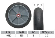
Puncture resistant, non-marking balloon cushion rubber on one-piece polyolefin hub with semi-precision bearings.
