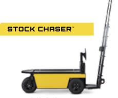
**STOCK CHASER** 1,000-lb Load Capacity, 2,000-lb Towing 24-Volt Drivetrain
